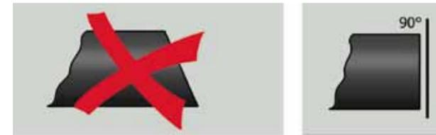
Cut the pipe using suitable tools, being careful to make the cut as perpendicular as possible with respect to the axle of the pipe itself.
