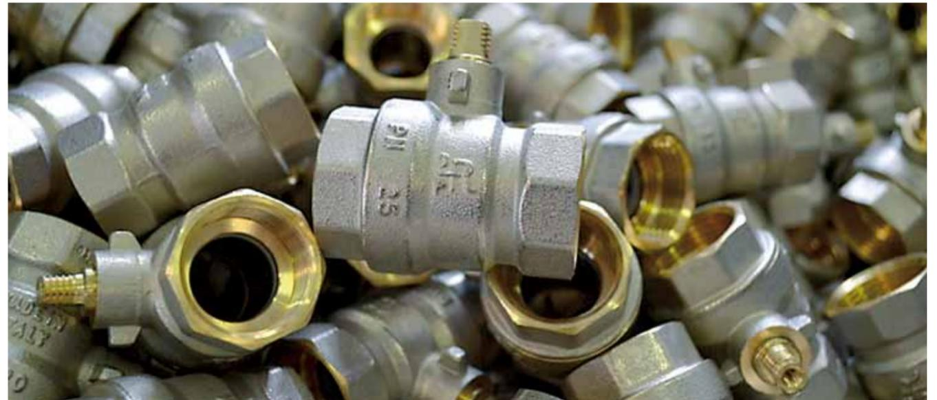
We get our products by hot molding the brass and the subsequent chip removal with transfer machines. All those items that do not require molding undergo the mono/multi mandrel machining. Ravani multilayer pipe is a product of the latest generation, made with advanced technologies in the processing of polyethylene polymers. It combines the advantages of a PVC pipe and those of a metal tube. It is flexible and robust, resistant to high pressure and high temperatures.
