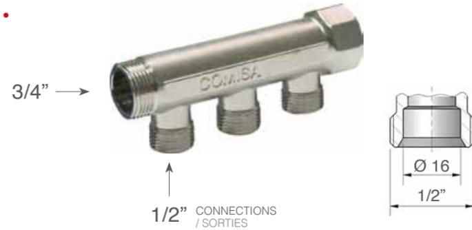
MANIFOLD 3/4" M x 3/4" F, CONNECTIONS 1/2" EURO - INTERNAL Ø 15 mm •
