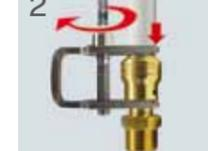
Through one complete rotation by using the Allen key tool and screw element are pressed together.
